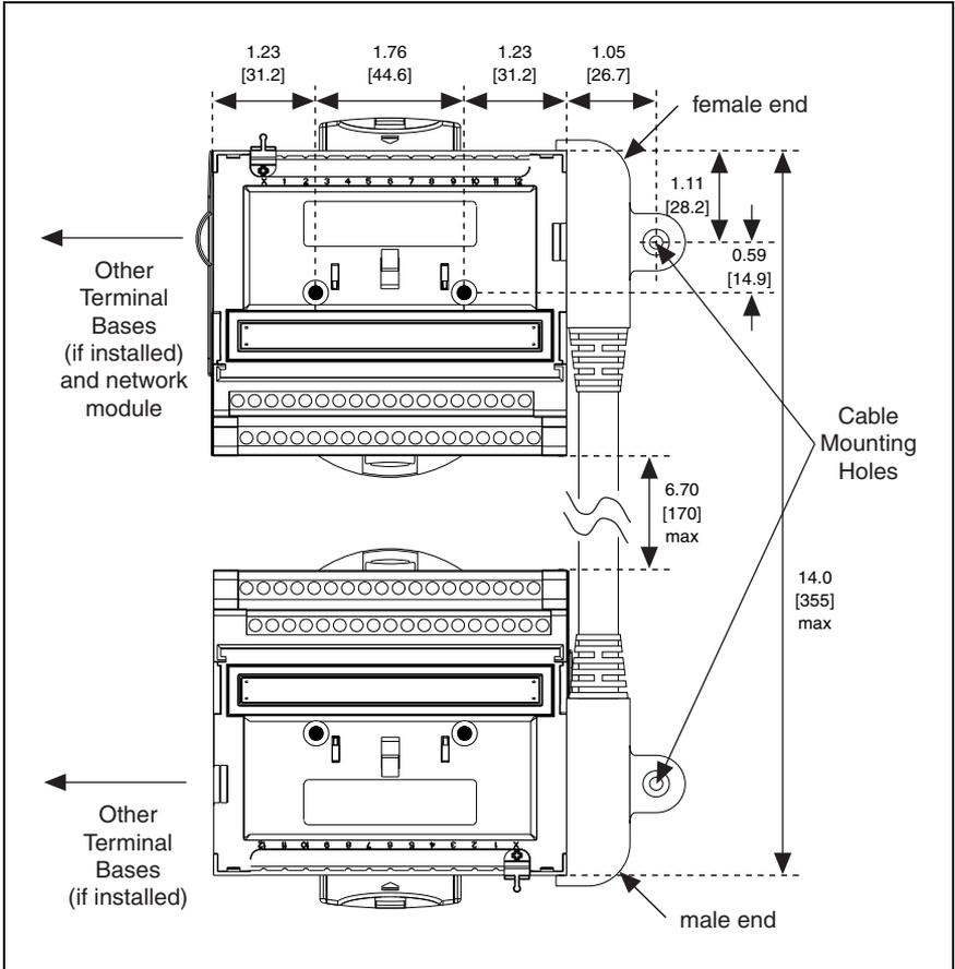
**Figure 2.** Mounting with Terminal Blocks Together
