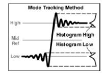
MINMax defines the 0% and 100% waveform levels as the lowest amplitude (most negative) and the highest amplitude (most positive) samples. See the figure below. This method is useful for measuring frequency, width, and period for many types of signals. However, this method is sensitive to waveform ringing and spikes and does not always accurately measure rise time, fall time, overshoot, and undershoot.
