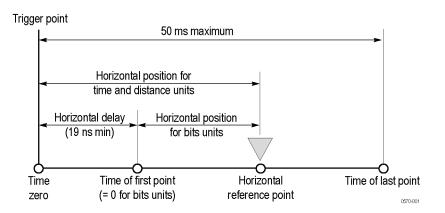
The position of the Mag timebase is constrained to be in the domain of the Main timebase. Changing the Main timebase position can affect the position of each Mag timebase, but a Mag timebase position cannot affect the Main timebase position.
