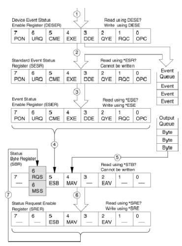
When an event occurs, a signal is sent to the DESER (1). If that type of event is enabled in the DESER (that is, if the bit for that event type is set to 1), the appropriate bit in the SESR is set to one, and the event is recorded in the Event
