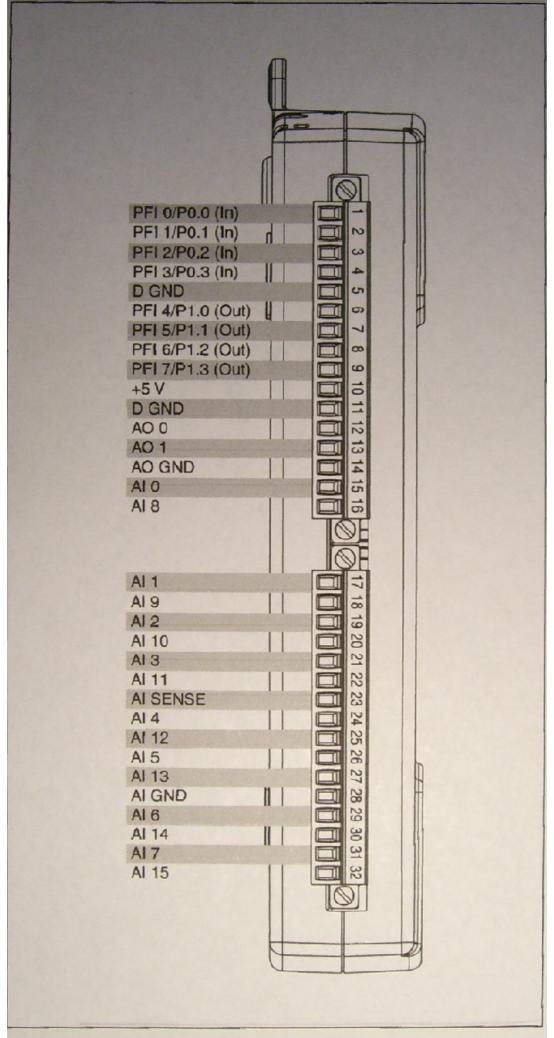
Figure 3. USB-6211/6215 Pinout
